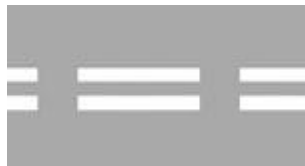
broken double white line
