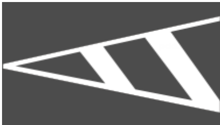
Islands that separate traffic flows in opposite directions
