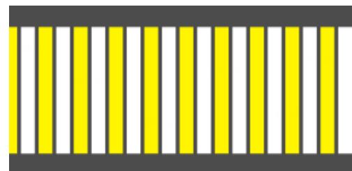
Marking of unregulated pedestrian crossings at ganger zone.
