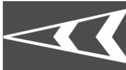
Islands that separate traffic flows in the same direction
