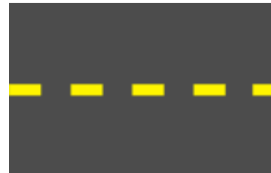
Designation of places where parking is prohibited
