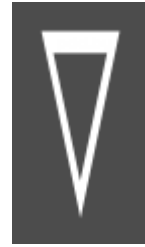
Approach designation to the place at intersection where the driver must stop to give way to other vehicles
