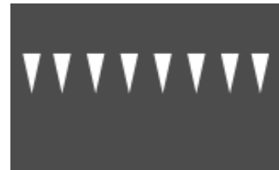
Marking the place at intersection where the driver must stop to give way to other vehicles
