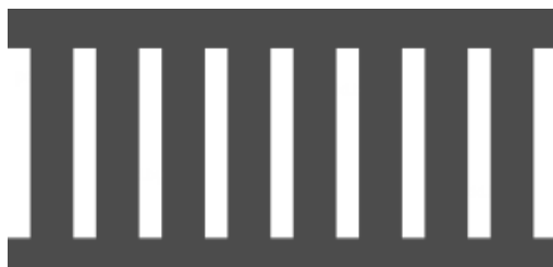
Marking of unregulated pedestrian crossings
