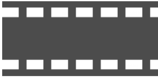
Marking of a pedestrians crossing regulated by traffic lights
