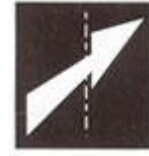
Warns about approach to the white continuous line
