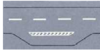
Bus stop bays
